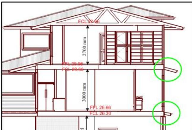
Figure 1 – Example of cantilevered eave awnings
