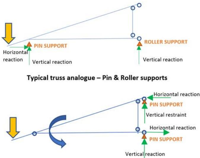
Typical truss analogue – Pin & Roller supports
