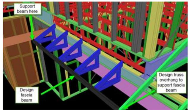
Figure 2 – Fascia beam support option where possible
